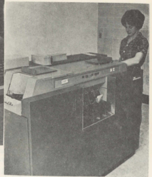
The central processor of the 1620 system is shown above. The control panel is in front and within this unit is the memory. In the photo on the right, the programmer, Miss Macmillan, operates the card reader and punch.
