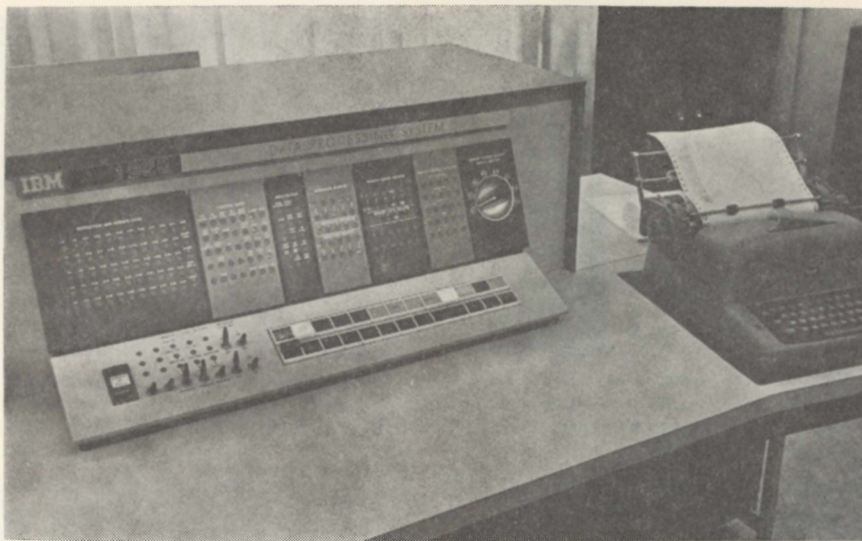
The central processor of the 1620 system is shown above. The control panel is in front and within this unit is the memory. In the photo on the right, the programmer, Miss Macmillan, operates the card reader and punch.
