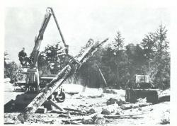
A knuckle boom loader is used to pile logs at the yard.
