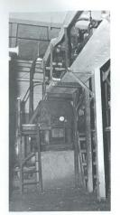
The installation of the bull screen rejectreclaim system in 1987 has resulted in 3 tons per day of slivers and coarse fibres from the groundwood mill being reclaimed for use in the sulphite plant. With some modifications to the system, a further 1.5 tons can be reclaimed daily.
