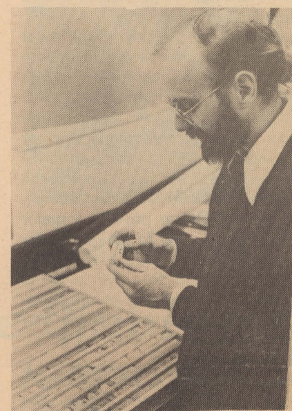
Dr. Pat Ryall , a research associate in the geology department, has a look at some of the drill core collected during his expedition to a seamount near the Azores group of islands. These rock columns, which were retrieved with a drill bit fitted with diamonds, show the composition of the ocean floor, which includes basalt and limestone. (Wilkins photo)
