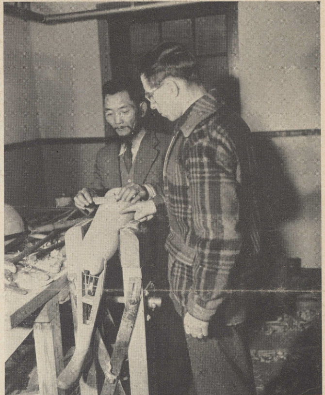
IN LIMB SHOP Presbyterian missionary Paul Kingsbury shows a Korean woodworker correct techniques for shaping the wooden socket of an A-K (above the knee) artificial leg.
