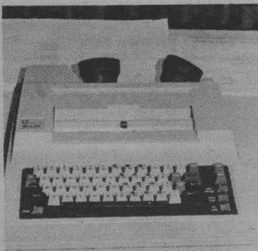
This "Silent 700" electronic data terminal weighs only 13 pounds and permits the scholar to record his material on Dalhousie's computer in the Killam Library while sitting at home by his telephone. [Carmichael Photo].
