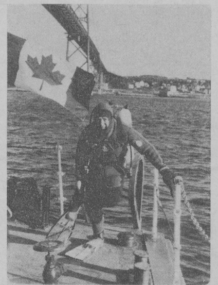
The Uni-suit is 1/4-inch foam neoprene nylon-packed on both sides, making the suit completely dry inside. An inlet and exhaust valve attached to it allows the diver to control his own buoyancy. The diver may also keep a layer of air in the suit, thus preventing "suit squeeze."
