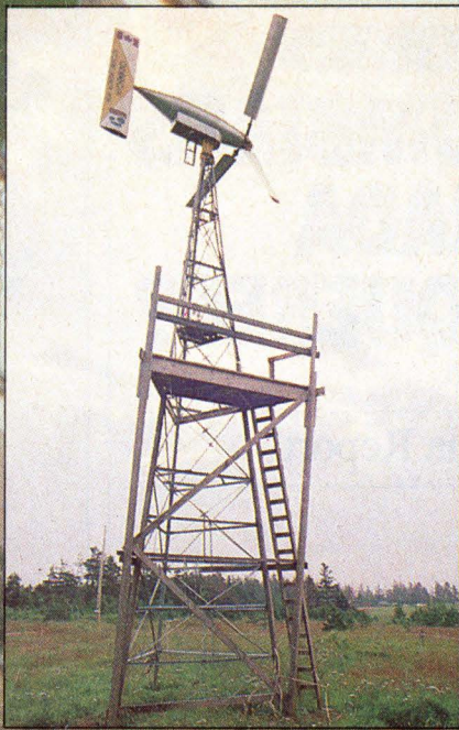
Far left: The Ark, powered by sun and wind, overlooks Northumberland Strait on Spry Point, P.E.I. Centre: Glass walls and roof solar collectors gather heat. The Ark is also a fish farm and tilapia will be raised in the round tanks. Near left: Six-kilowatt windmill generates power for household appliances. Below: Even in midwinter, Nancy Willis, David Bergmark, who run the Ark, and their children Meredith and Chris, can pick fresh chard and other vegetables from the greenhouse for supper.
