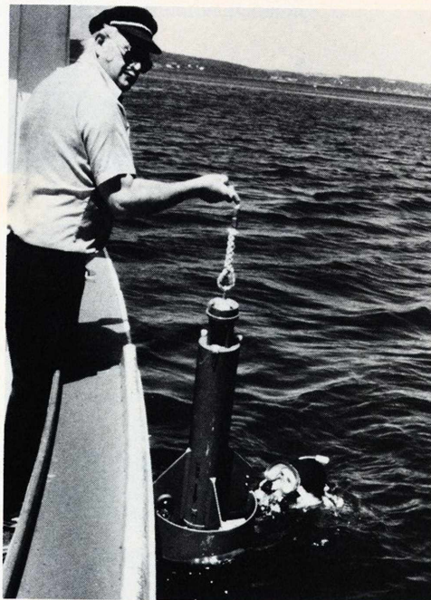
Diver recovering current meter
