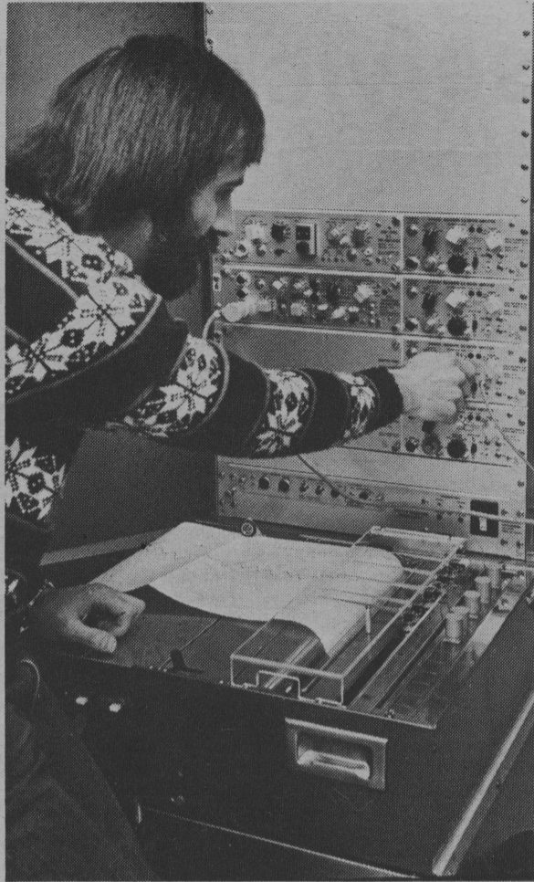
Dr. John Reeves and his assistant Sandy Hodson use the Grass model 7D Polygraph to measure heart rate, GSR, respiration, peripheral blood flow and EMG muscle potential. The machine makes a permanent record of the data collected.
