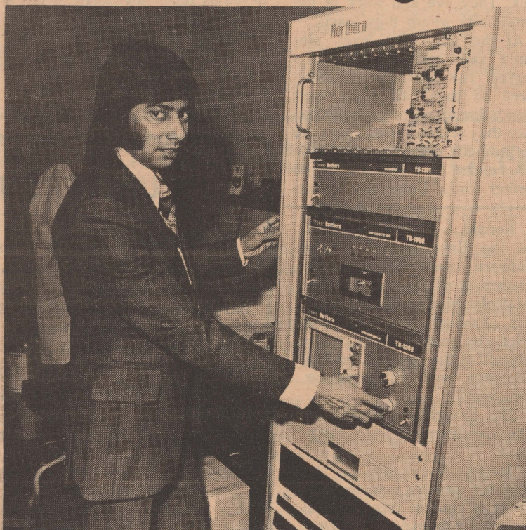
Dr. Chattopadhyay, a member of the Dalhousie Speakers Bureau, demonstrates sophisticated computer-assisted gamma-ray spectrometer system. [John Donkin, A/V Services]
